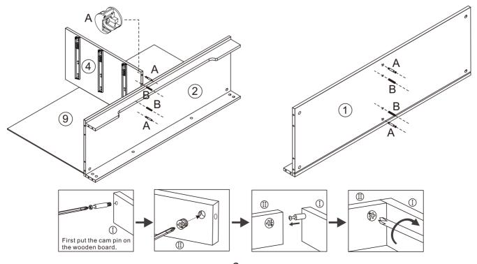
1. Attach panel 1 to panel 4 with parts A and B.
